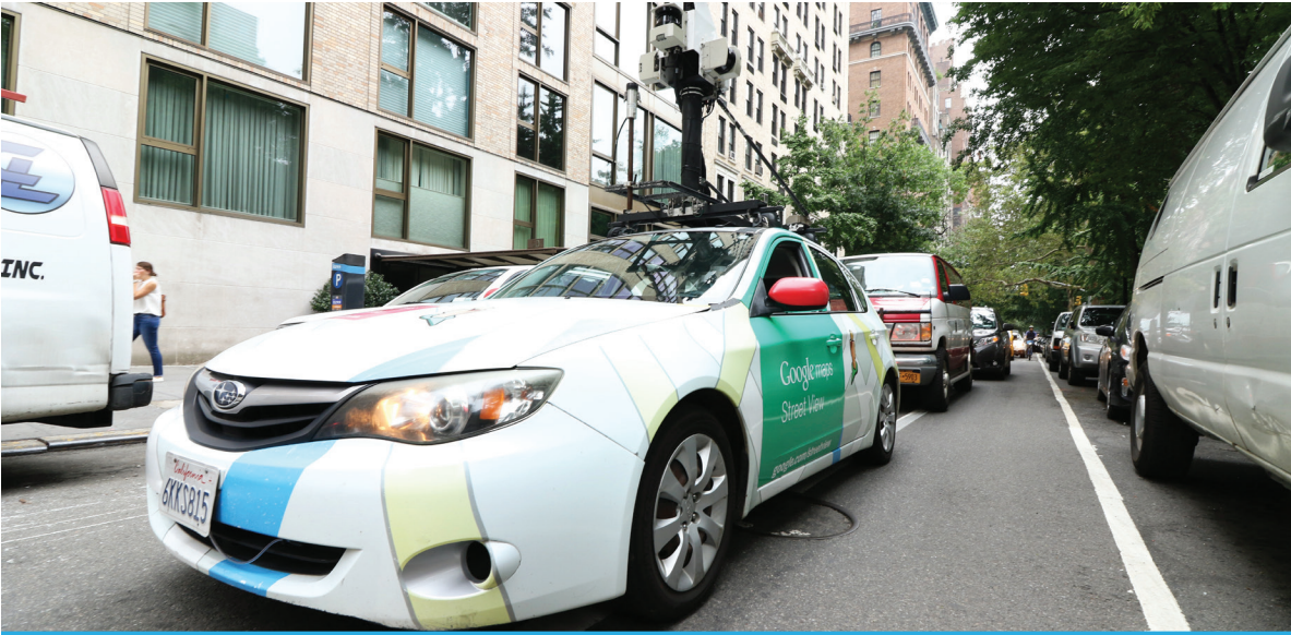
EDF teamed up with Google Earth Outreach to pinpoint methane leaks under our streets and sidewalks from natural gas pipes.
