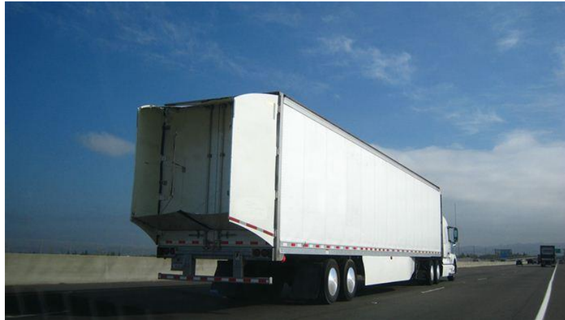
Figure 2: Aerodynamic Side Skirt and Boat Tail
