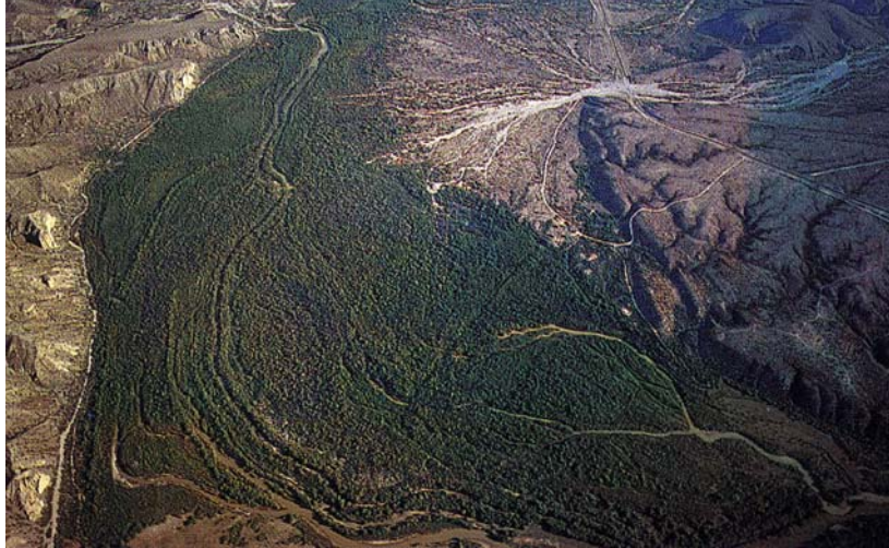
Figure 8 - A myriad of small channels as a result of sediment aggradation and saltcedar establishment characterize much of the Forgotten Reach. Areas like these comprise thousands of acres and are responsible for attenuation of flows. (USGS, 1996)
