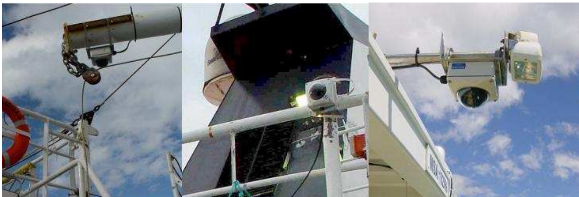
Figure A2 CCTV camera installations on three different fishing vessels. Each camera has a mounting bracket and stainless steel mounting straps.
