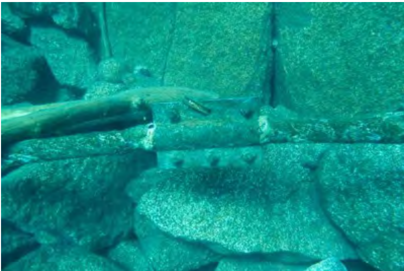
(E) Part of a broken anchor on the cable near Rubicon. April/March 2022. Lake Tahoe, California.
