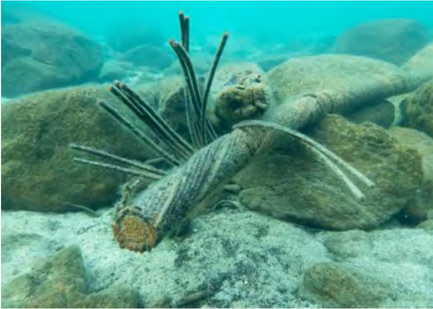
(G) Severed end of 1920's cable in Emerald Bay. May 2021, Emerald Bay - Lake Tahoe, California.
