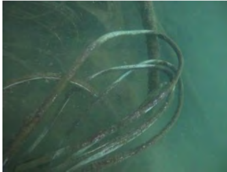
(G) Close up of bare lead from abandoned cables. Site LP 4.1. August 2022, Lake Pend Oreille, ID.
