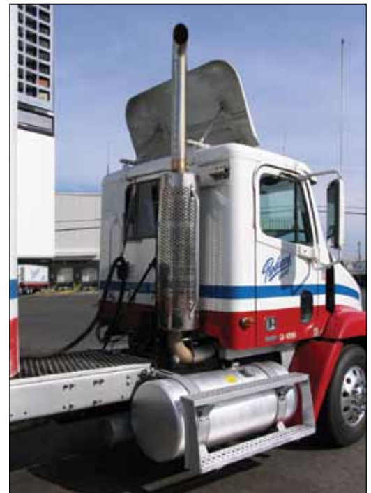
Providing incentives for add-on technologies, like this retrofitted exhaust pipe, helps existing engines run cleaner.
